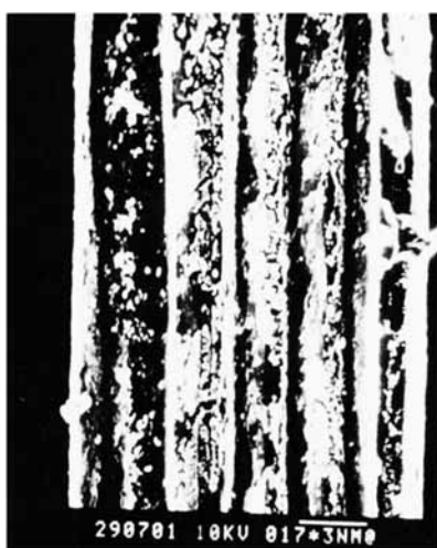
Figure 8 Electron microphotograph of 23.1% MMA grafted tossa jute.
