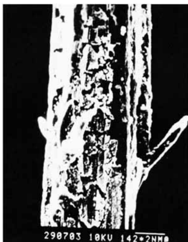
Figure 11 Electron microphotograph of 31.8% grafted tossa jute (MMA:AN = 50:50).
